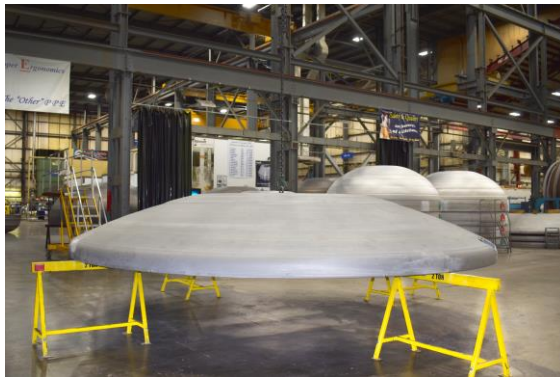
Core stage fuel tank dome
